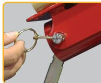
Quick-release clevis style pins for easy crane assembly without tools.
