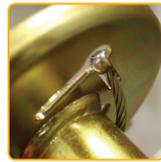
Swaged ball fitting allows you to quickly attach or remove the wire rope from the winch - Wire rope remains attached to submerged pumps, etc., while the crane is stored or moved to a new location.
